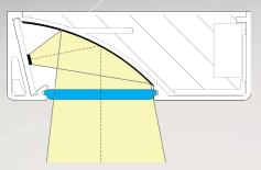
Using a 98% efficient reflector, light from the LED sources inside the housing diffuse inside the mixing chamber in order to create evenly distributed illumination. Patent Pending
