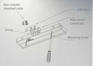
Side wiring door and captive mounting screws for installation ease
